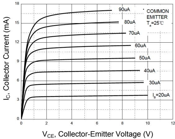
Figure 1. Static Characteristic
