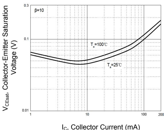
Figure 4.  $V_{CESat}$  —  $I_C$
