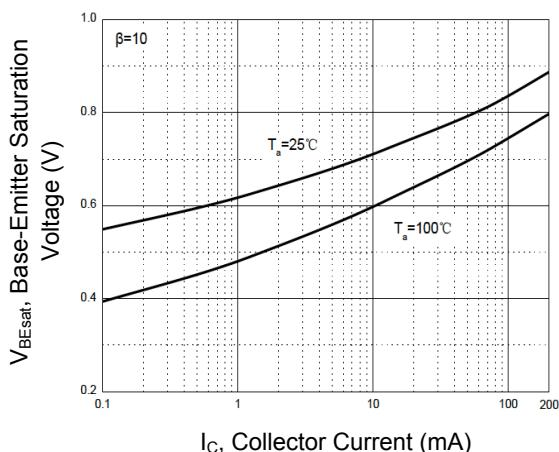
Figure 3.  $V_{BEsat}$  —  $I_C$
