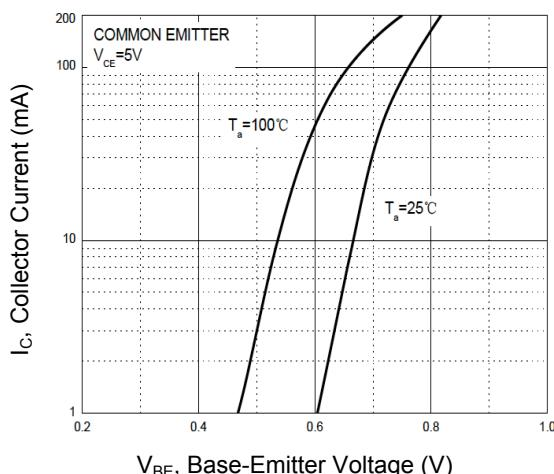
Figure 5.  $I_C$  —  $V_{BE}$
