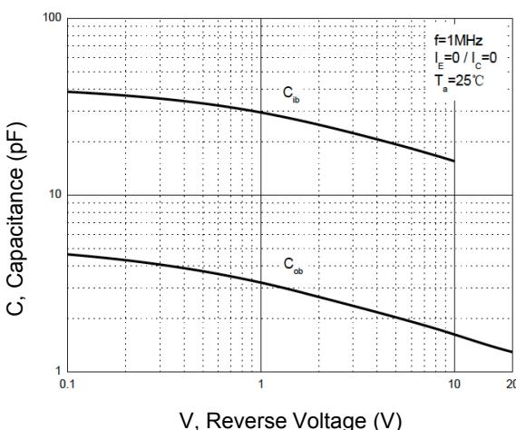
Figure 6.  $C_{oe}/C_{ib}$  —  $V_{CB}/V_{EB}$
