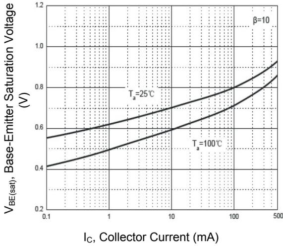
**Figure 3. Base-Emmitter Saturation Voltage vs. Collector Current**
