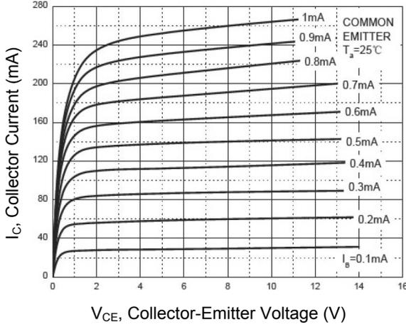
**Figure 1. Static Characteristic**
