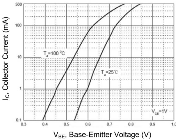
**Figure 5. Collector Current vs. Base-Emmitter Voltage**
