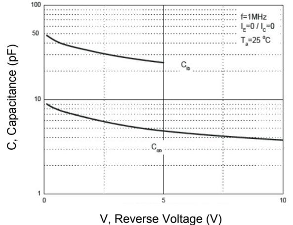
**Figure 6. Capacitance Characteristics**
