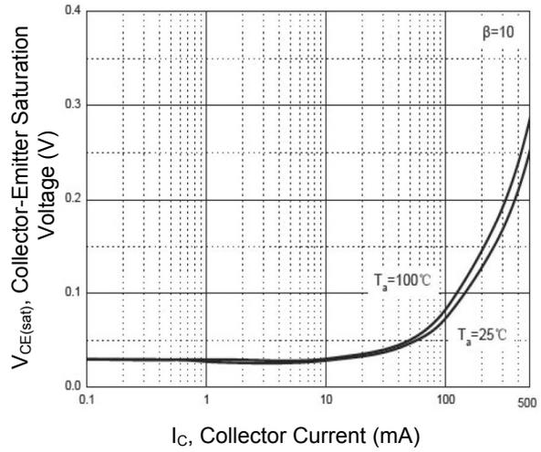
**Figure 4. Collector-Emmitter Saturation Voltage vs. Collector Current**
