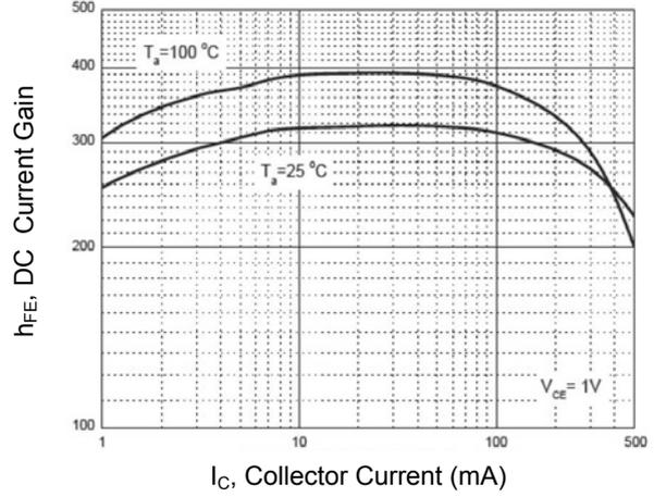
**Figure 2. DC Current Gain vs. Collector Current**
