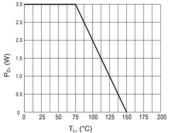
Figure 6. Steady State Power Dissipation
