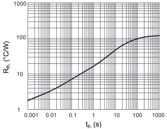
Figure 4. Typical Transient Thermal Impedance
