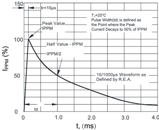
Figure 3. Pulse Waveform
