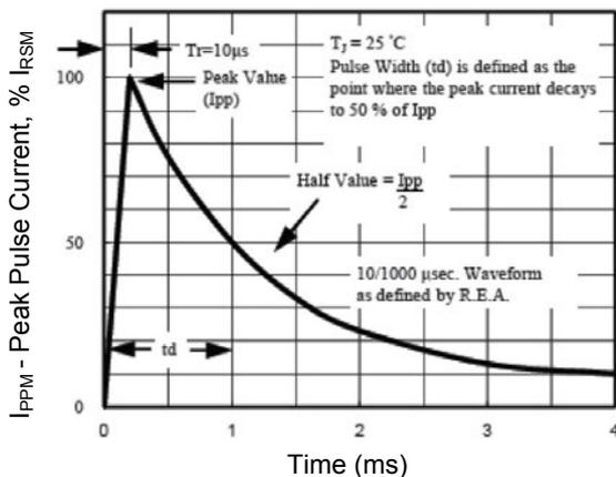
Figure 5. Pulse Waveform
