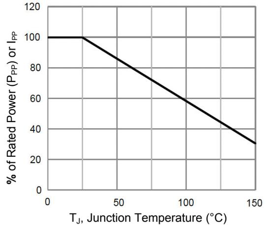
**Figure 4. Pulse Power or Current vs. Initial Junction Temperature**
