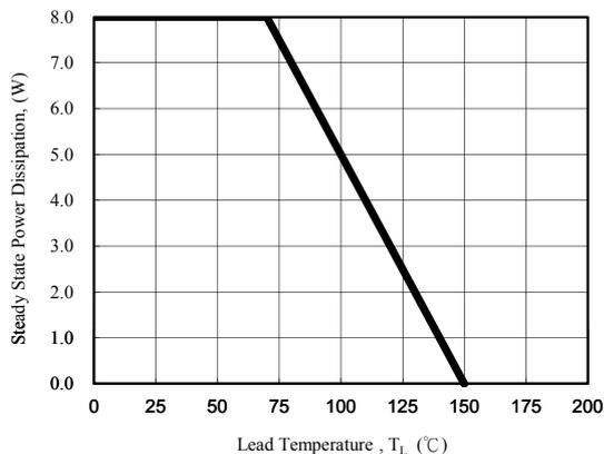
Fig. 3 - Steady State Power Derating Curve
