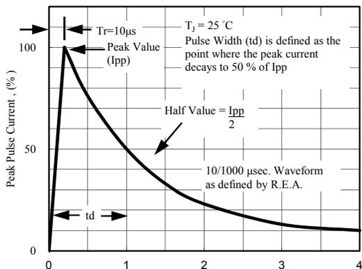
Fig. 5 - Pulse Waveform
