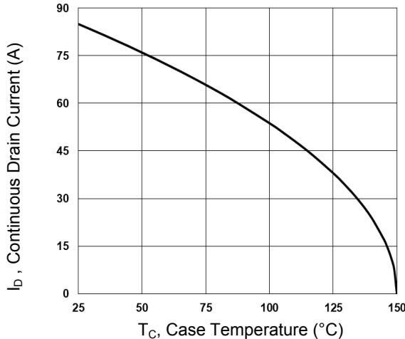
Figure 1. Continuous Drain Current vs. T<sub>c</sub>
