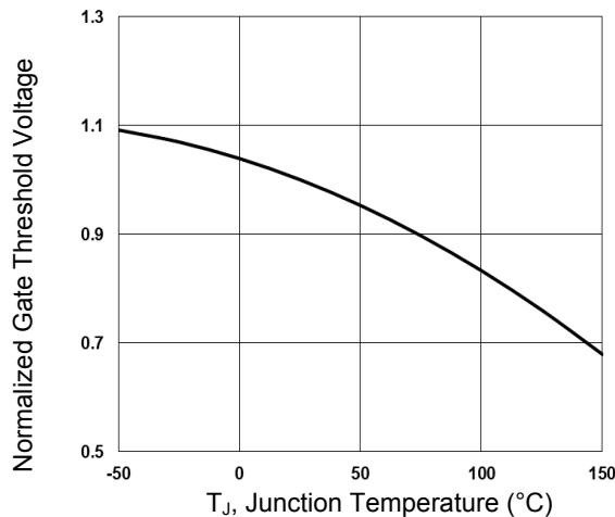
Figure 3. Normalized V<sub>th</sub> vs. T<sub>j</sub>
