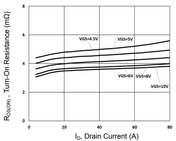
Figure 6. Turn-On Resistance vs. I<sub>D</sub>
