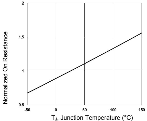
Figure 2. Normalized R<sub>DS(ON)</sub> vs. T<sub>j</sub>
