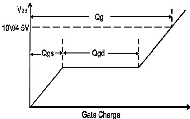
**Figure 11. Gate Charge Waveform**
