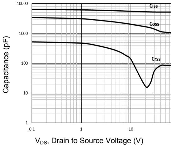
**Figure 7. Capacitance Characteristics**
