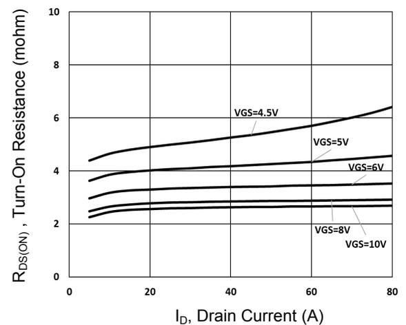
**Figure 6. Turn-on Resistance  $R_{DS(ON)}$  vs  $I_D$**
