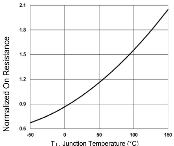
Fig.2 Normalized R<sub>DS(ON)</sub> vs. T<sub>J</sub>
