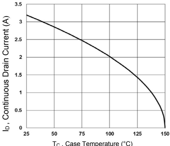
Fig.1 Continuous Drain Current vs. T<sub>c</sub>
