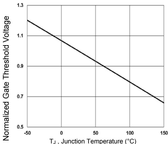
Fig.3 Normalized V<sub>th</sub> vs. T<sub>J</sub>
