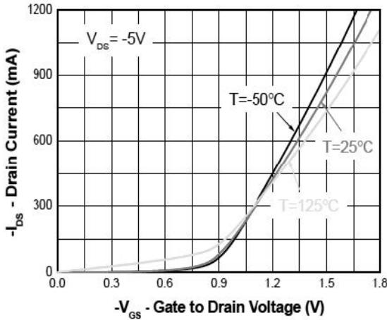
Figure 11. Transfer Characteristics
