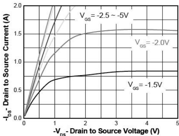
Figure 1. Output Characteristics
