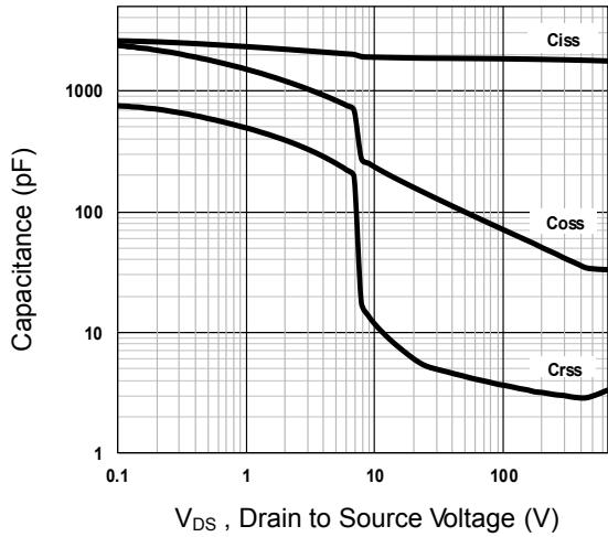
Figure 7. Capacitance Characteristics
