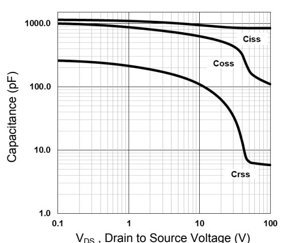
Figure 6. Capacitance Characteristics
