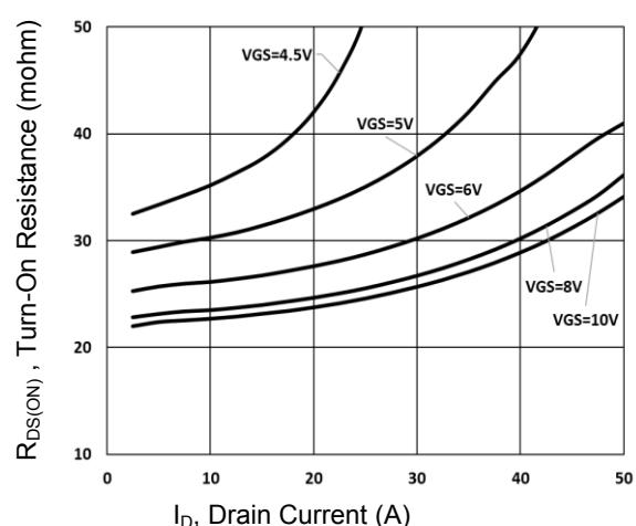
Figure 6. Turn-on Resistance vs. I<sub>D</sub>
