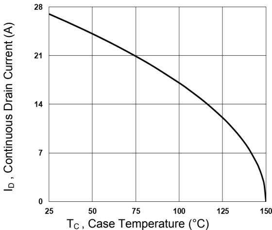
Figure 1. Continuous Drain Current vs. T<sub>c</sub>
