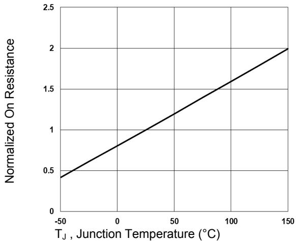
Figure 2. Normalized R<sub>DSON</sub> vs. T<sub>j</sub>
