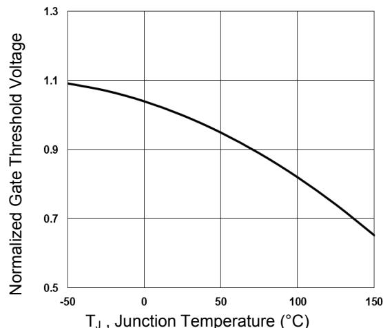
Figure 3. Normalized V<sub>th</sub> vs. T<sub>j</sub>
