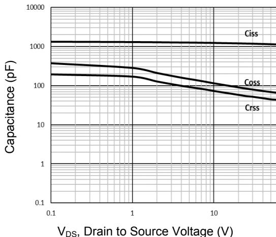
Figure 7. Capacitance Characteristics
