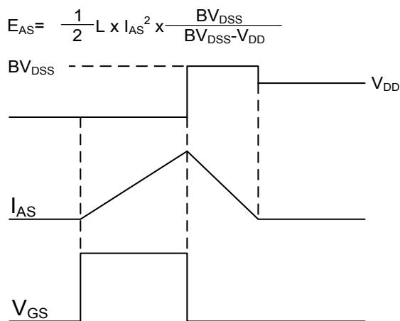
Figure 11. E<sub>AS</sub> Waveform
