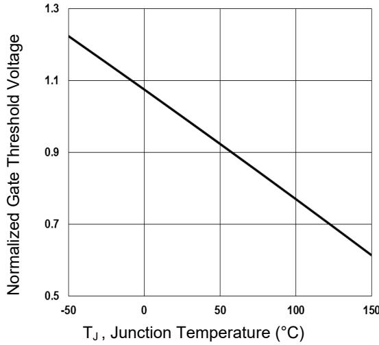
**Figure 3. Normalized V<sub>th</sub> vs. T<sub>j</sub>**
