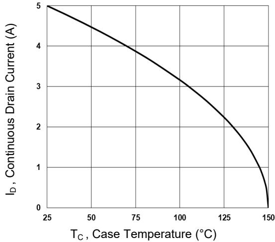
**Figure 1. Continuous Drain Current vs. T<sub>c</sub>**
