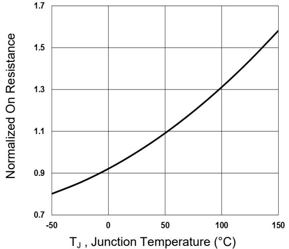
**Figure 2. Normalized R<sub>DSON</sub> vs. T<sub>j</sub>**
