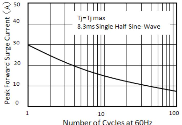
Figure 2. Maximum Non-Repetitive Peak Forward Surge Current
