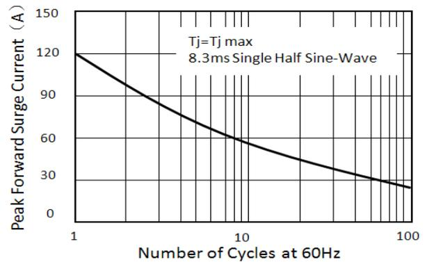
Figure 2. Maximum Non-repetitive Peak Forward Surge Current
